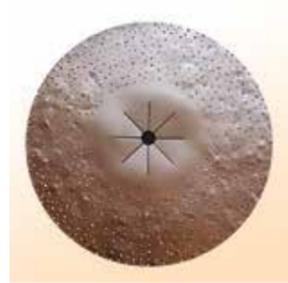
**Disc with electrodeposited tungsten coating**
